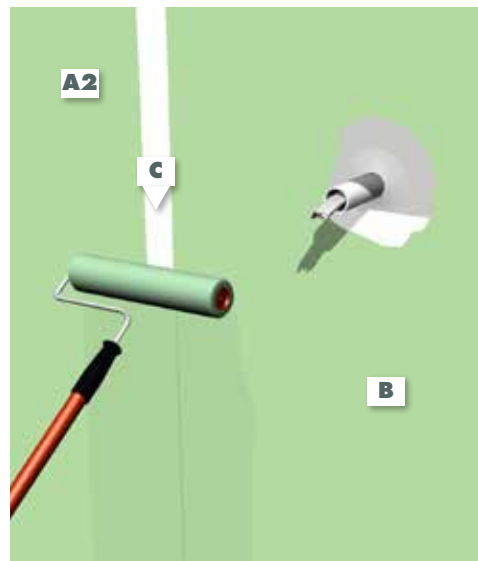
Joint treatment for MVIS Air Barrier over sheathing
